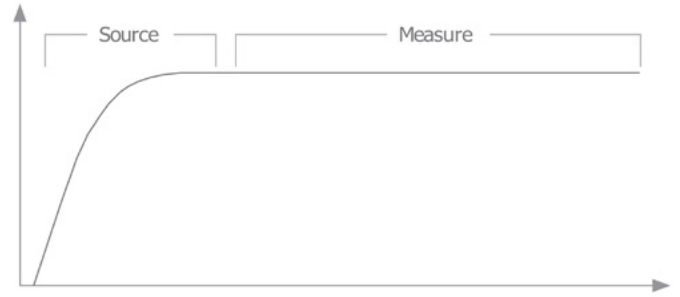
FIGURE 4 Illustration of the Aperture Time of an SMU with Respect to a Sample Signal
