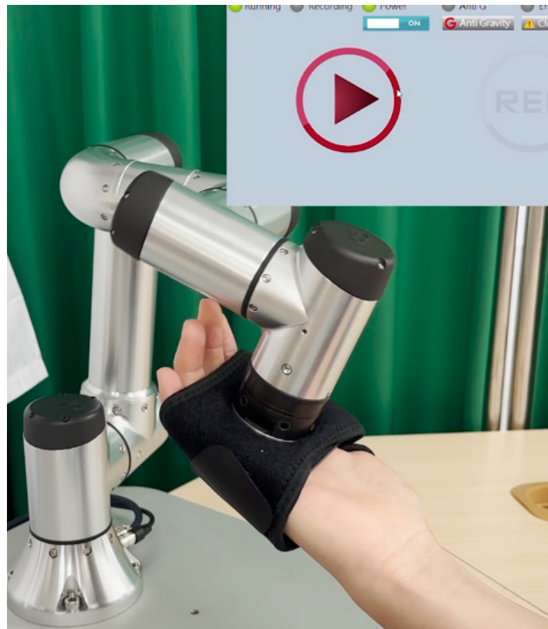
The S0 performs repetitive exercises to assist in upper limb physiotherapy. (Image: Chieftek.)
